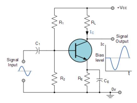
This is the simplest type of Class A power amplifier circuit. It uses a single-ended transistor for its output stage with the resistive load connected directly to the Collector terminal. When the transistor switches "ON" it sinks the output current through the Collector resulting in an inevitable voltage drop across the Emitter resistance thereby limiting the negative output capability.
