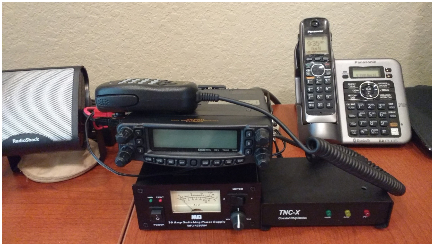
Yaesu FT-8800 with Bluetooth TNC-X GPS from cell phone running APRSDroid
